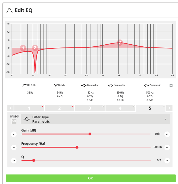
Fig. 27 Window "Output – Edit Equalizer"
