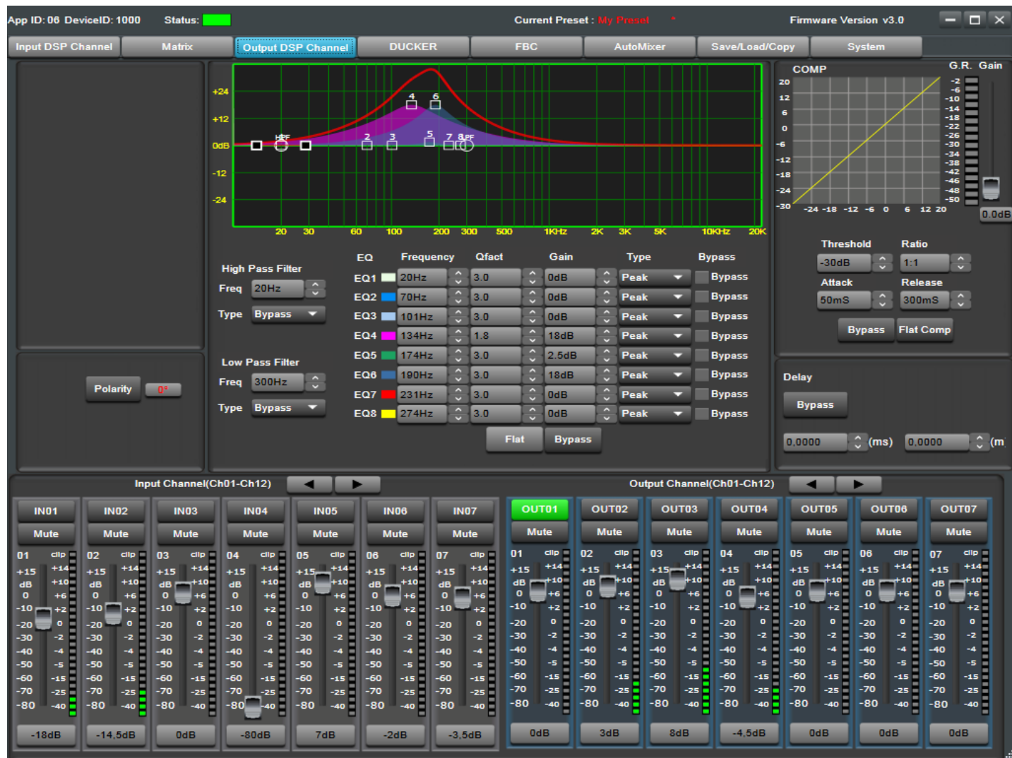
Fig. 22 View "Output DSP Channel"
